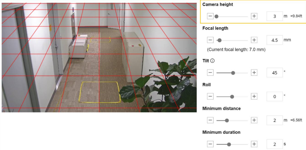
Image 17. Camera height configured at 3 meters
