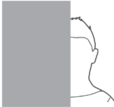
Image 8. (Undesirable condition) When a head is occluded more than 25% from left to right.
