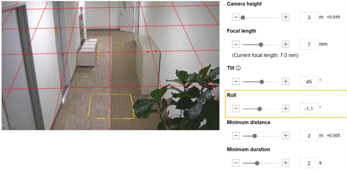
Image 19. Camera rotation angle set up at -1.1 degrees
