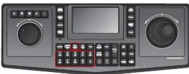
If you have layouts saved, you can select these on the monitor screen by pressing the layout number on the keypad then the LAYOUT/SEQ. button
