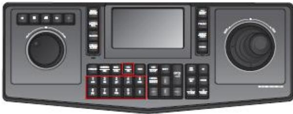
Cameras can be selected using the number key of the camera then the CAM button – cameras can be assigned numbers under the configuration page in SSM
