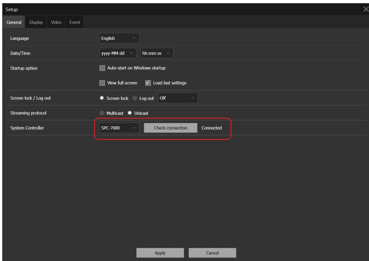
Select the SPC-7000 keyboard under the General – System Controller section and check connection – Connected should be displayed if the keyboard is connected correctly
