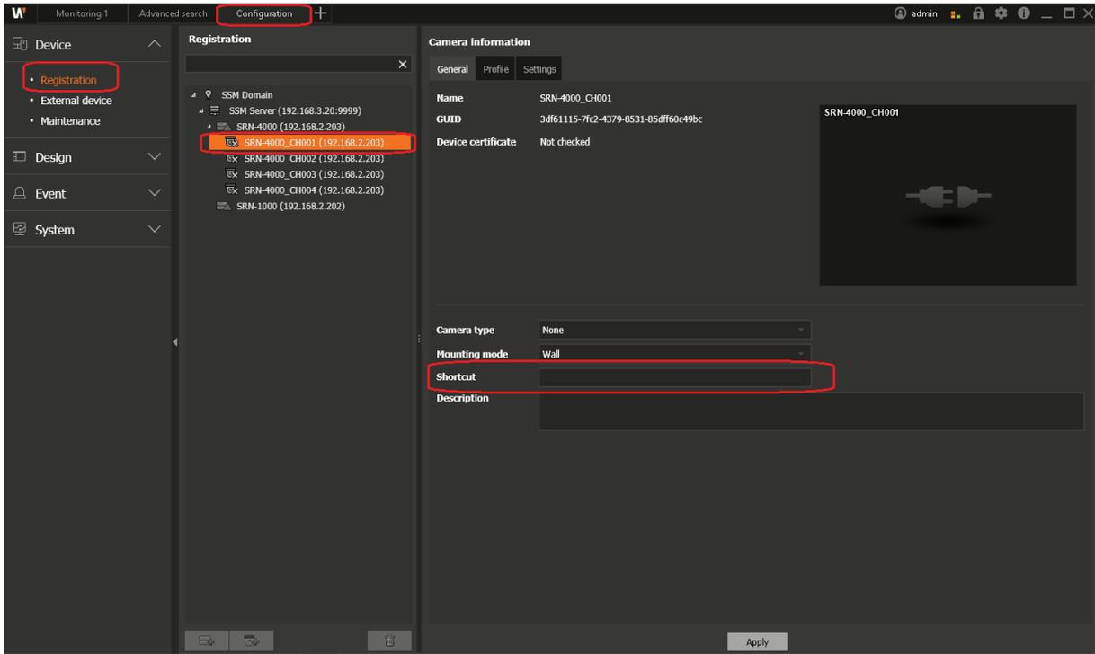
The shortcut section is where a camera number can be assigned in SSM
