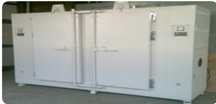
<Fig. 8. Drying chamber>
