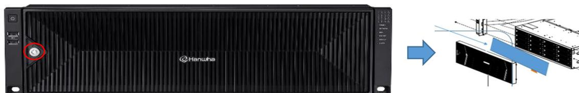
(2) Type having no locking system: There is a Dust Filter at the back of removed Front Case when pressing a red circle part.
